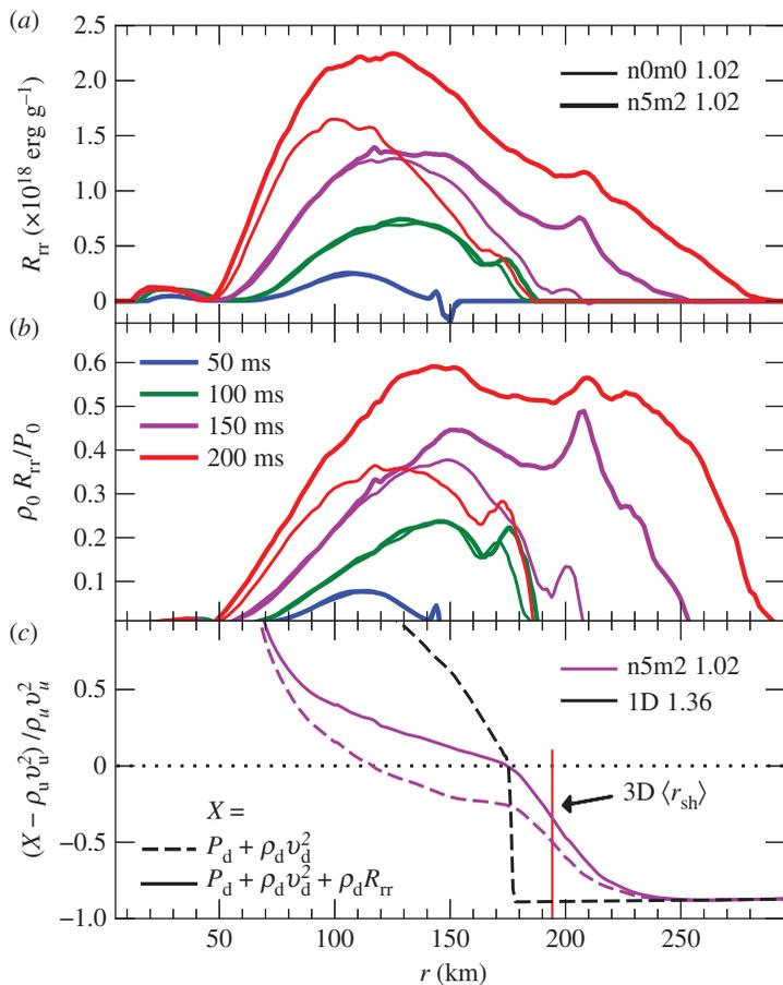
**Figure 4.** Quantities demonstrating the strength and importance of turbulence in 3D CCSNe: (a) radial–radial component of the Reynolds stress; (b) turbulent pressure scaled to the background thermal pressure; (c) excess in the shock jump conditions (cf. equation (7.1)) scaled to the upstream ram pressure. In this figure,  $\rho_0$  and  $P_0$  are the spherically averaged density and thermal pressure, and  $r_{\text{sh}}$  is the average shock radius. From Couch *et al.* [108].
