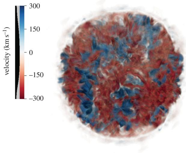
**Figure 5.** Radial velocity field from the 3D massive star simulation of Couch *et al.* [108] just prior to the onset of core collapse. This image shows the Si-burning-driven convection in the shell surrounding the iron core, around 1500 km in radius.
